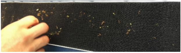
The idea behind the freezing mechanism was that the flowers would be sprayed with water and then rolled on a very cold surface. We thought in the same way that your tongue sticks to a metal pole in the winter that the leaves of the flower would stick to the cold surface. Then, by rolling it on the cold surface, you the leaves would rip off the flower.
