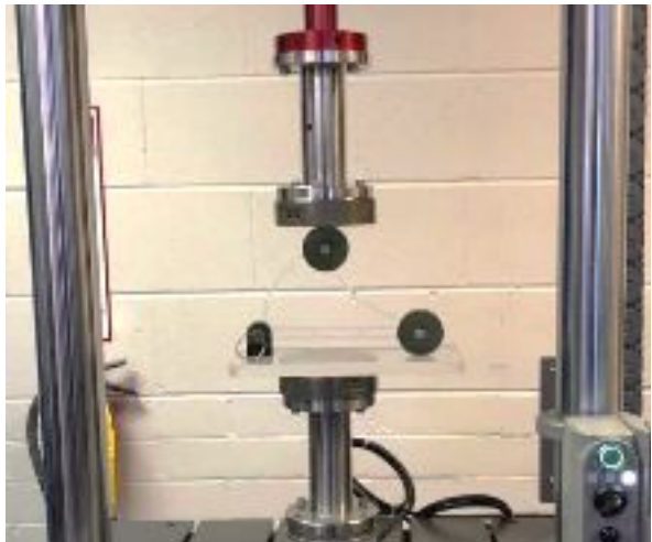
Figure 14 (left): Structure #1 in Instron Machine ready for testing
